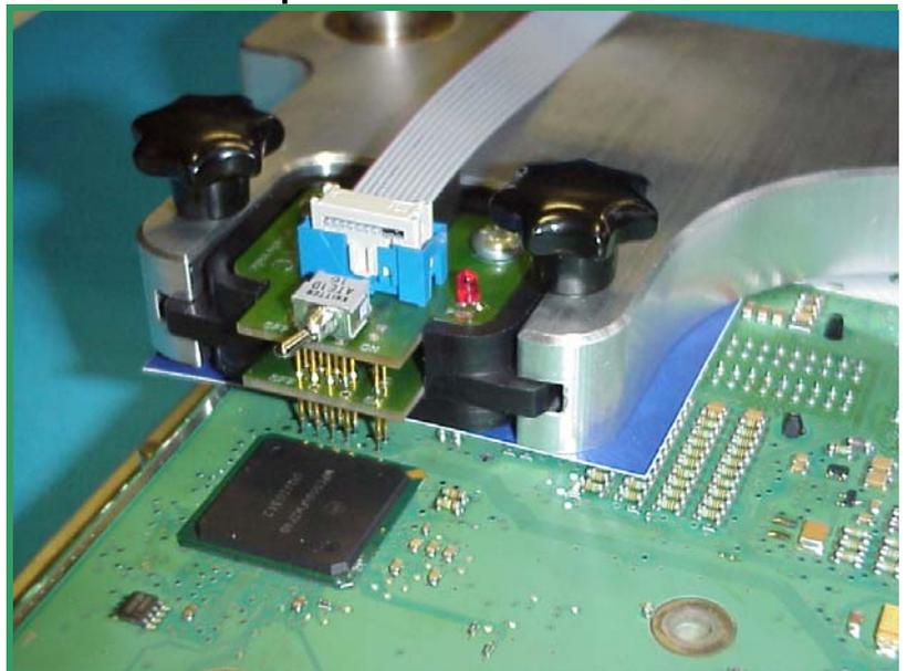
**Pict. B:** The BDM143 probe contacting the pads.
