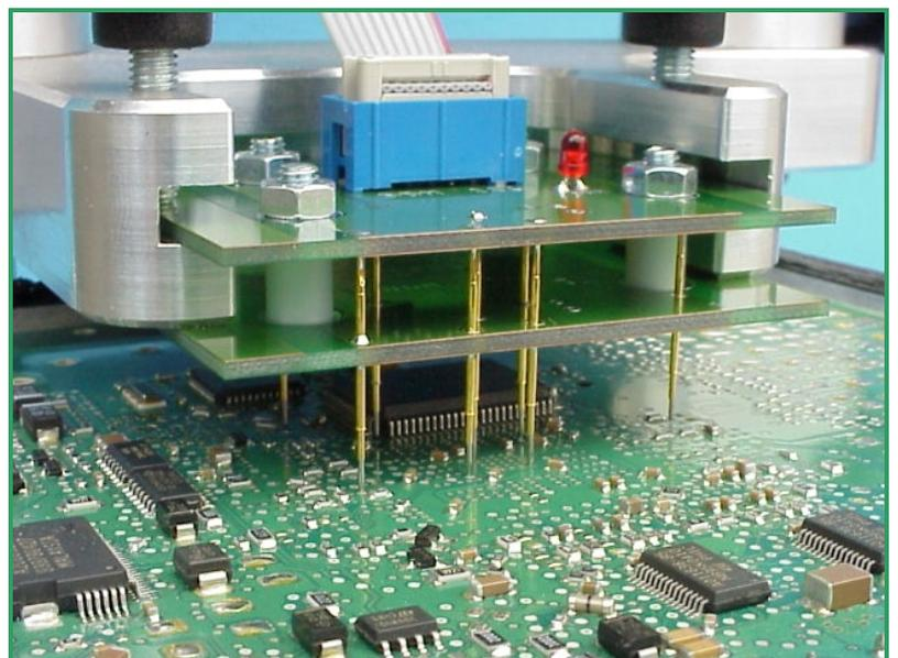
**Pict. C: The tips of the spring contact probes should reach a spring travel of 2mm minimum for best contact conditions**
