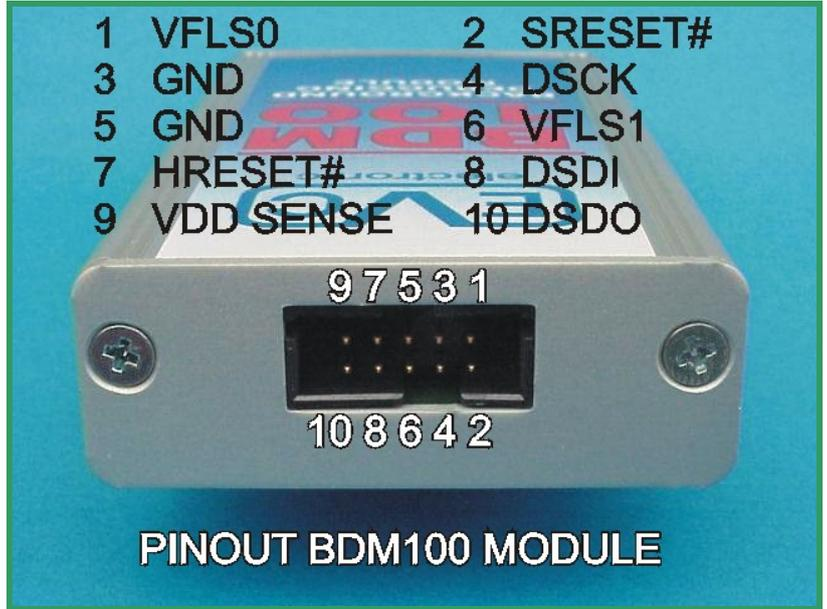
**Pict. A:** The pinout of the 10way pin header
