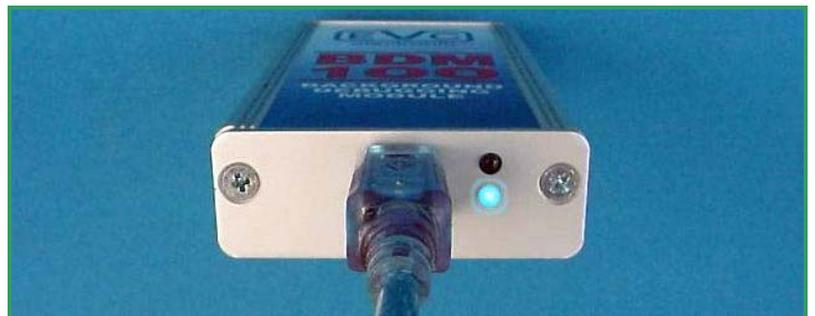
**Pict. A: The BDM100 Module is always connected to the USB cable first.**
